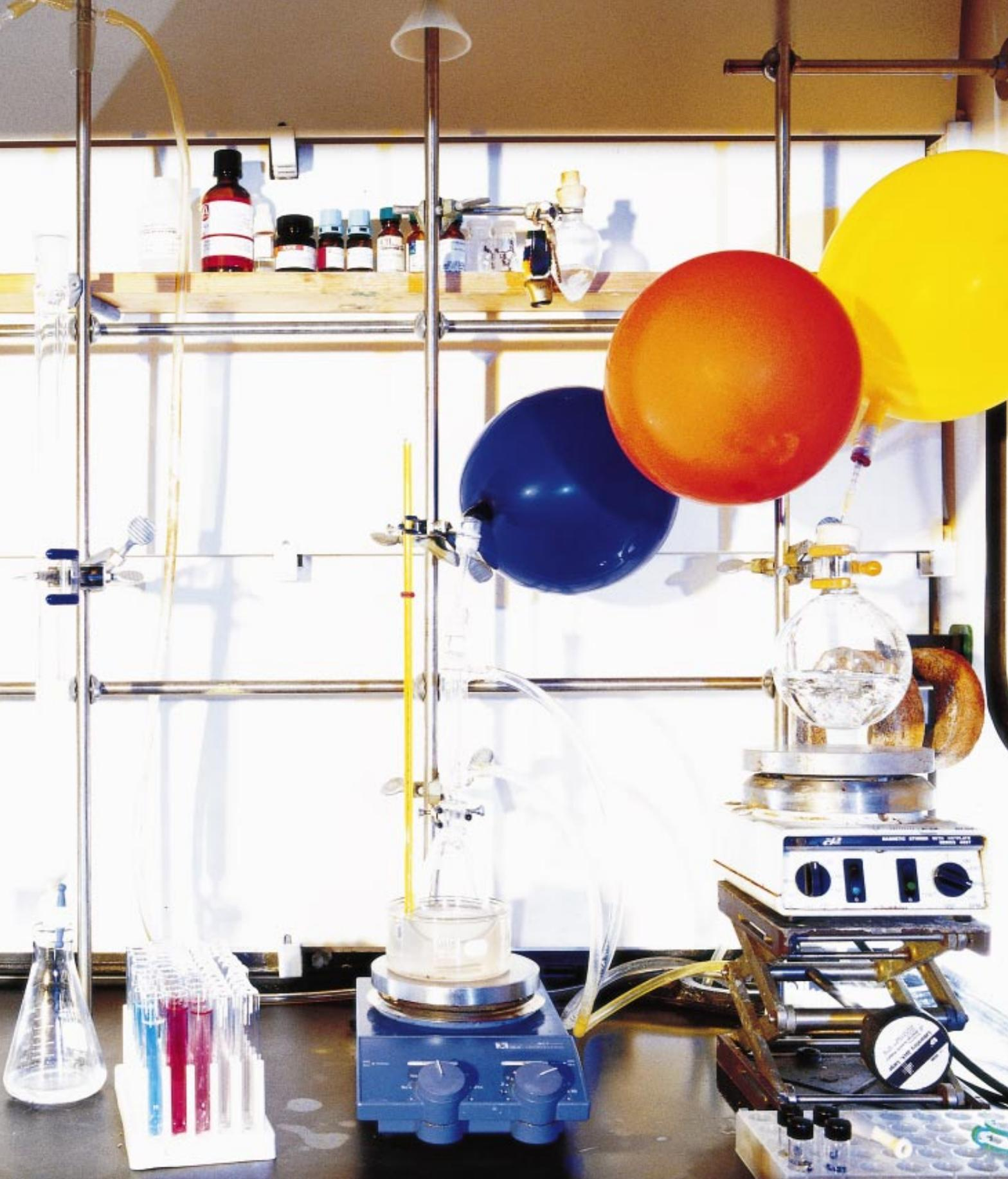
**COMPOUNDS** are mixed in the chemist's workspace under the fume hood. In the setup to the left, organic molecules are being purified. In the two to the right, reactions occur in the presence of argon gas, which is in the balloons and which protects sensitive molecules from oxygen and water in air.
